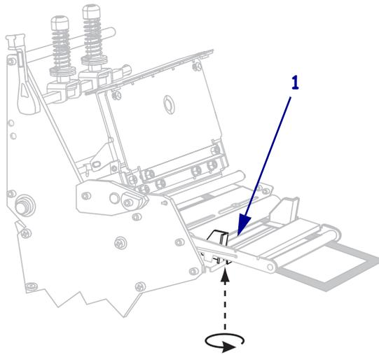
10. Push down the printhead assembly (1), and then rotate the printhead-open lever (2) clockwise until it locks into place.
