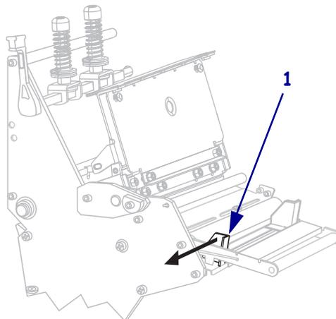
7. If your printer includes a media dancer assembly (1), thread the media under the media dancer assembly roller. For all printers, thread the media under the media guide roller (2) and then the upper media sensor (3).
