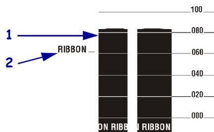
**Media Sensor Profile (Figure 29)** The media sensor readings are shown as bars and flat areas on the sensor profile. The bars (1) indicate gaps between labels (the web), and the low areas (2) indicate where labels are located. If you compare the sensor profile printout to a blank length of your media, the bars should be the same distance apart as the gaps on the media. If the distances are not the same, the printer may be having difficulty determining where the gaps are located.
