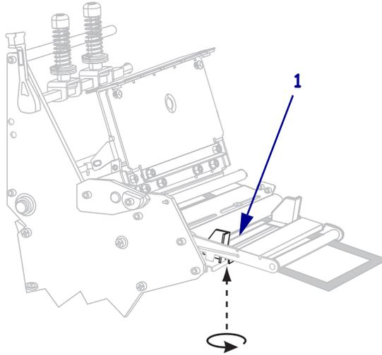
21. Push down the printhead assembly (1), and then rotate the printhead-open lever (2) clockwise until it locks into place.
