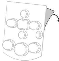
2. Carefully align the cover over the keypad. Press to make the cover adhere to the printer.
