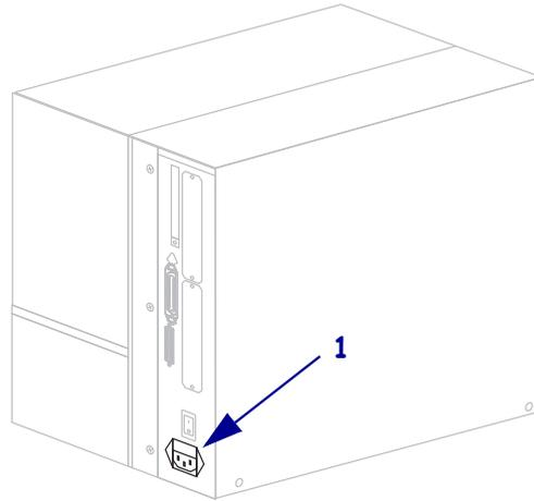
3. Plug the other end of the power cord into a power outlet near the printer.
