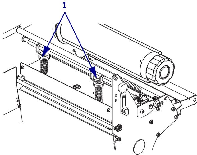
2. Slide the toggles until they provide even pressure on the media. For extremely narrow media, position one toggle over the center of the labels, and decrease the pressure on the unused toggle.
