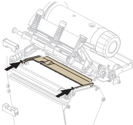
4. Rotate the front of the snap plate upward.
