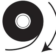
4. Place the roll of ribbon on the ribbon supply spindle. Push the roll back as far as it will go.
