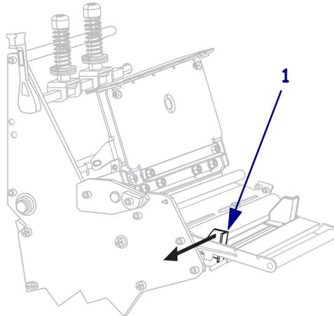
6. If your printer includes a media dancer assembly (1), thread the media under the media dancer assembly roller. For all printers, thread the media under the media guide roller (2) and then the upper media sensor (3).
