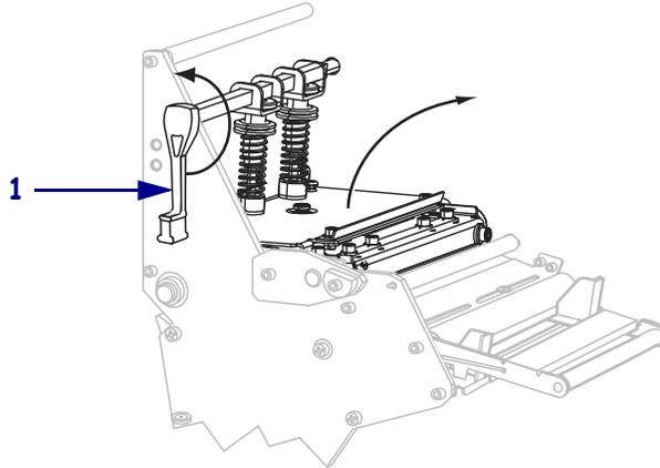
9. Loosen the thumb screw (not visible from this angle) that is located on the bottom of the outer media guide (1).
