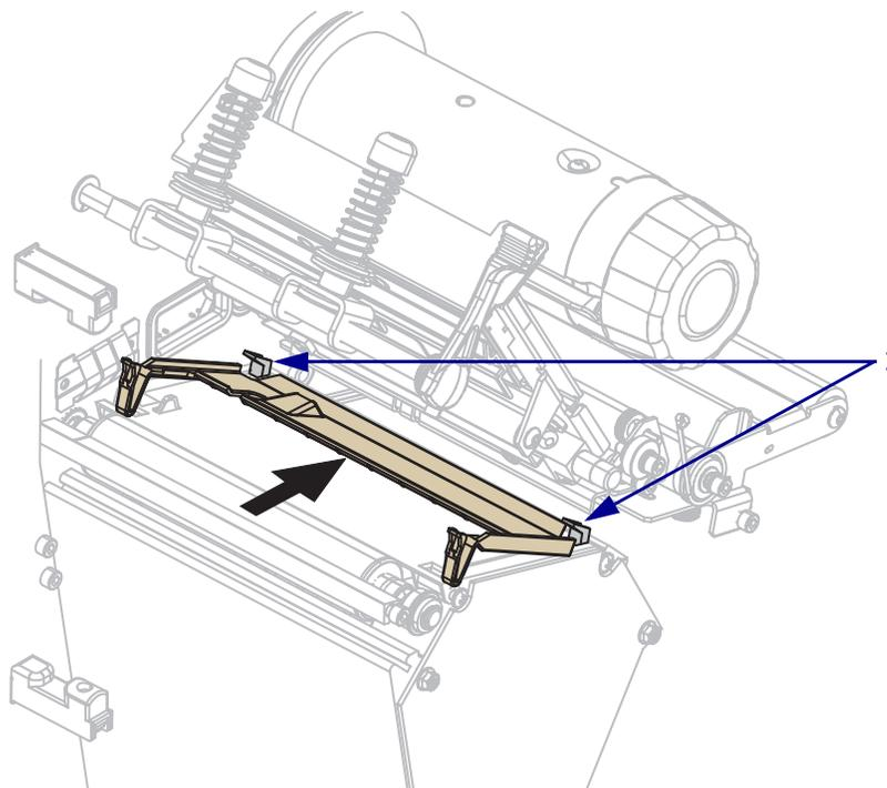
8. Press down on the tabs to lock the snap plate into place.
