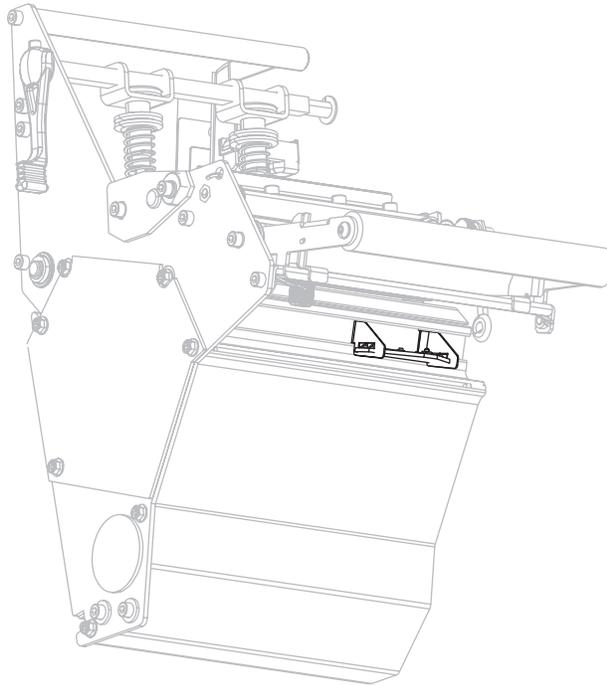
2. Slide the lower sensor until it is under the upper media sensor. Use the light that shines from the lower sensor to help align it with the upper sensor. Gently pull the wires as needed (wires should have a little slack).
